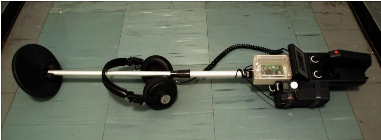
**Figure 5 Customized metal detector – “The Heavy Metal Detector”**
